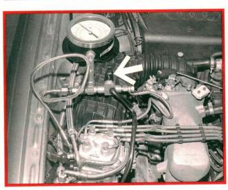
Measuring KE-Jetronic Differential Pressure
