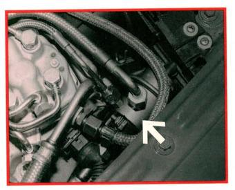
Measuring KE-Jetronic System Pressure
